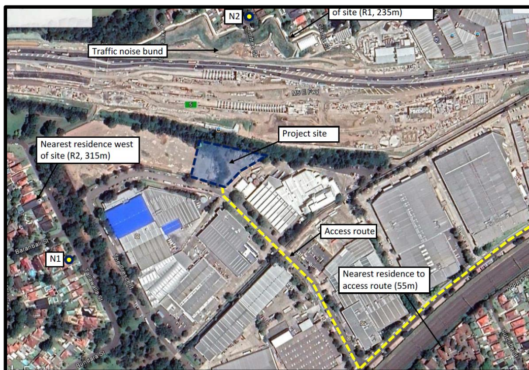
Figure 25: Location of the two noise loggers N1 and N2 (courtesy Spectrum Acoustics, 2019)
